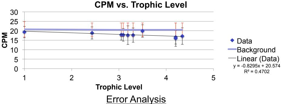
Aside from the background radiometric levels of my house and the inherent triggering energy limitation of our Geiger counter, there were few sources of intrinsic error to consider. One consideration is how fresh the seafood was; this information was nearly impossible to determine, but could have a huge effect on measure radioactivity (indeed, the time since death is the determining factor in <sup>14</sup>C dating, where the half-life is in thousands of years, not around 30 as for  $^{137}$ Cs).
